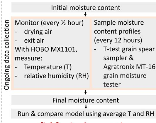
Fig 4. Overview of measurements
