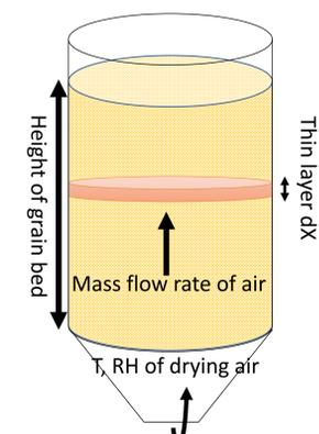
Fig 2. Thin-layer drying model inputs
