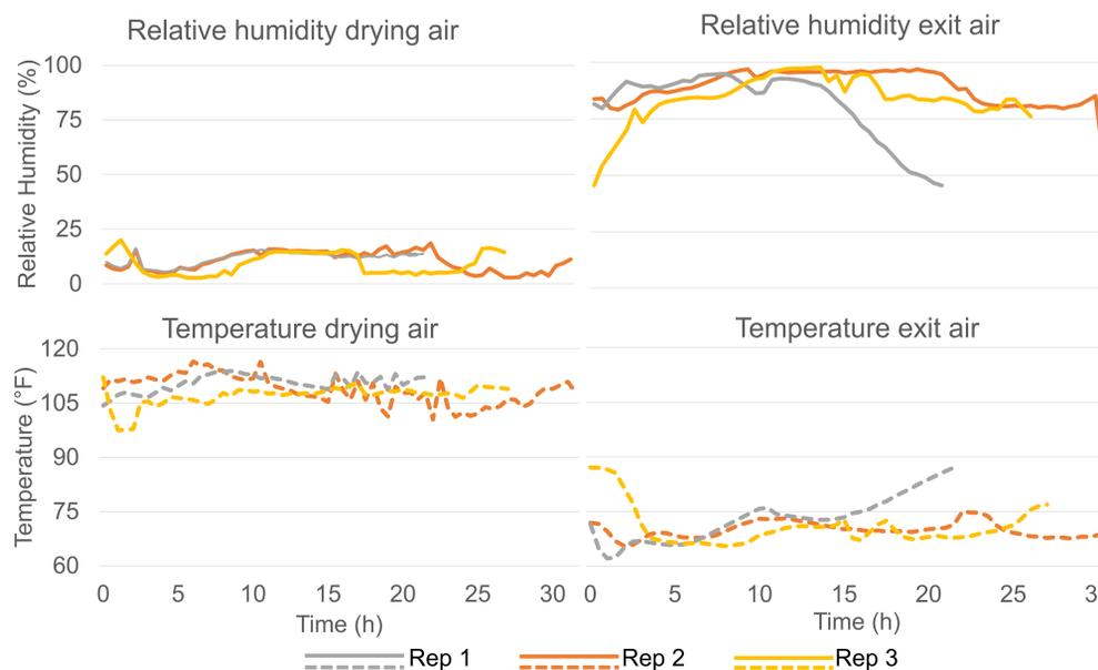
Fig 5. Temperature and relative humidity of drying and exit air throughout drying period
