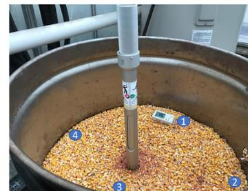
Fig 3. Moisture content profile collected from center and 4 sides
